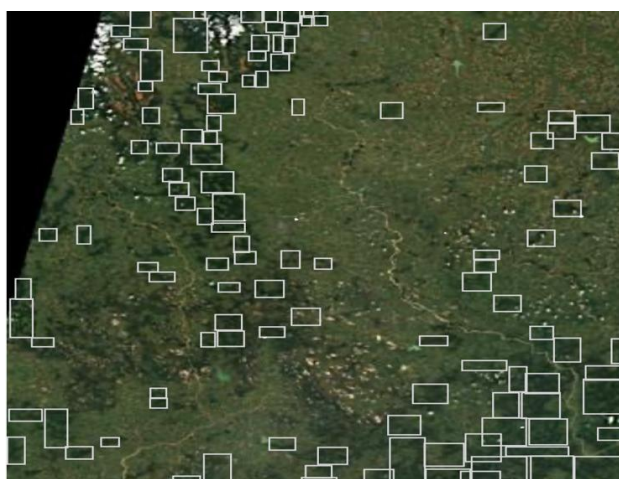
Fig 3: Tree canopy detection in the Sentinel 2 MSI imagery using QGIS
