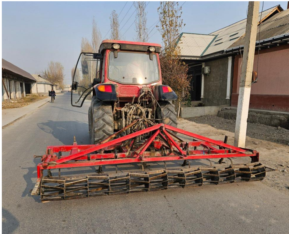
Figure 2. View of a chisel cultivator equipped with a developed improved plank roller during operation.
