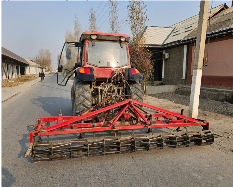
Figure 1. General view of the chisel cultivator equipped with the developed improved plank roller.
