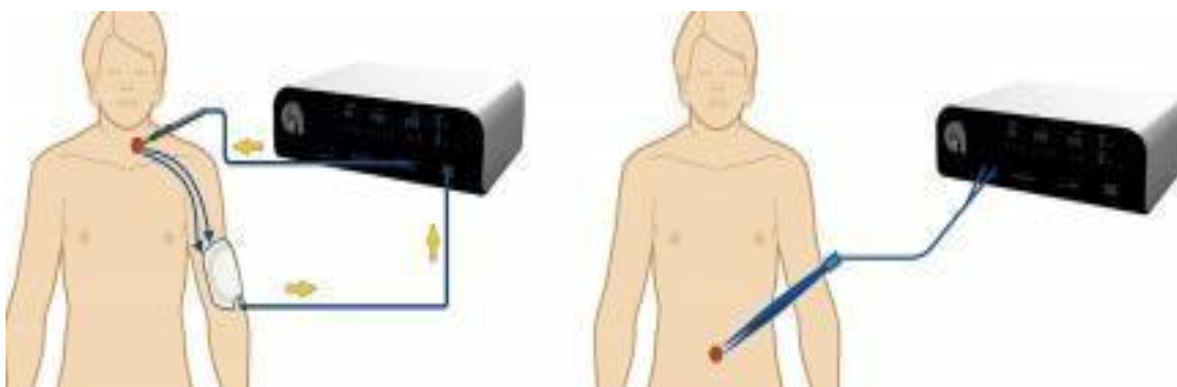
Figure 2-5 Working diagram of electrosurgical unit.
