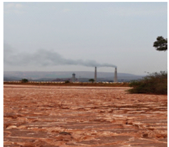
Fig:- 11 and 12 NALCO Solid WASTAGE (Red mud Pond water after dried to hard red soil.)
