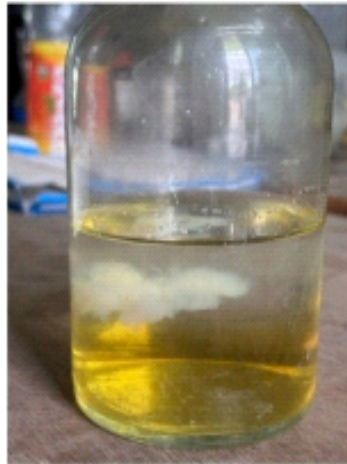
Fig :- Water sample of Ash pond showing cloudy formation
