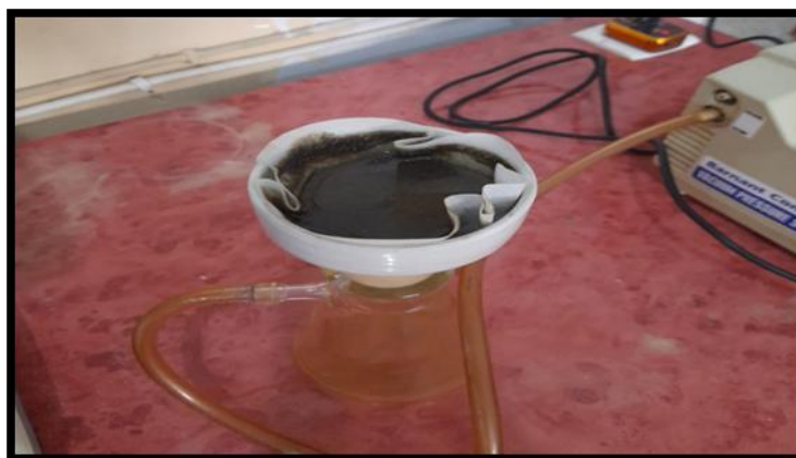
Figure (1): Filtering method using Oryza sativa powder
