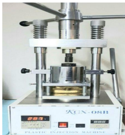
Figure (3): Plastic Injection Machine, Special Flask at temperature 287°C
