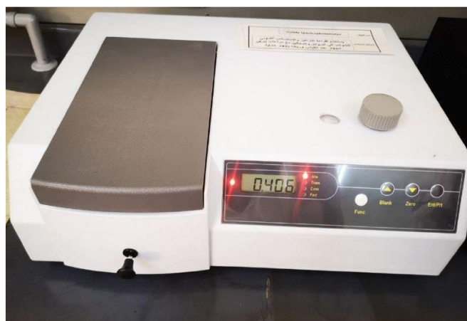
Figure (8) cuvette with the fluid inside the Visible spectrophotometer tester
