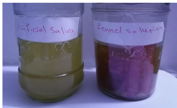
Figure (5): Soaking flexible samples in fennel herb solution
